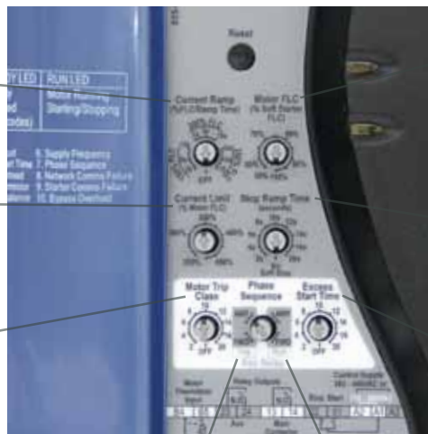
CSXi control panel
