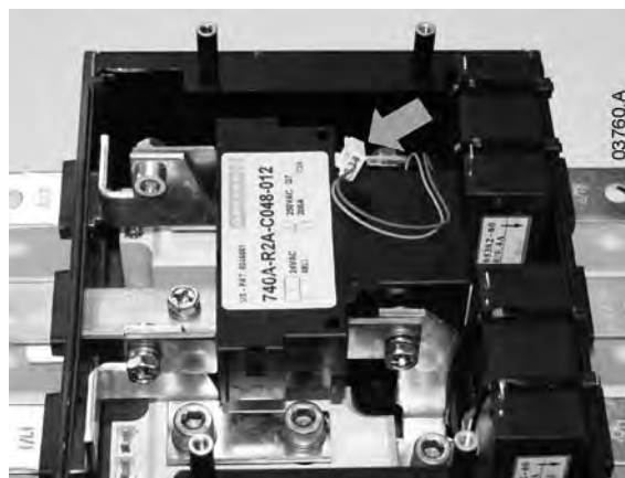
Figure 3: Bypass relay control wires (75 kW ~ 110 kW models)
