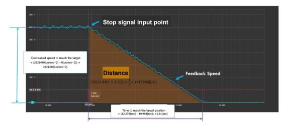
The target position is equal to the area of the distance shown in the figure above. If you want to stop the motor for approximately 2 seconds after inputting STOP signal while the motor is running at 300 rpm in index mode, you can calculate Quick Stop Deceleration as follows.
