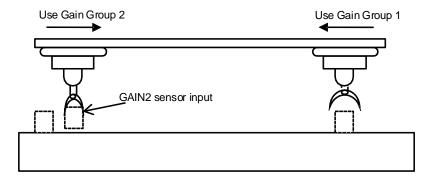
This is one of the gain adjustment functions and is used to switch between Gain Groups 1 and 2. You can reduce the time required for positioning through gain conversion.
