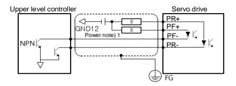
**Note 1)** When using 5[V] power: Resistance R = 100-150[ $\Omega$ ], 1/2[W]
