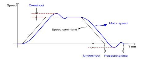
You make these settings in the P/PI control switch mode (0x2114). See the details below. Switching to P control by PCON input takes precedence over this setting.
