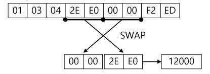
Be cautious with parsing for a 2 byte register since 1 byte for each of the upper and lower parts is swapped. For example, '2E E0 00 00' is swapped and converted into a decimal number, 12000.
