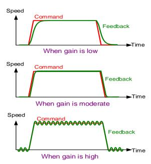
The error between the position command and the current position is multiplied by the proportional gain, and the result is converted to a velocity command. The higher the gain, the better the responsiveness of position control. In many cases, a value that is 0.2~0.5 times of the speed proportional gain is applied for a stable structure.
