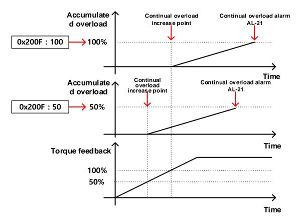
The default value is 100. If torque feedback exceeds 100 [%], accumulated overload keeps accumulating, causing an occurrence of the continuous overload alarm (AL-21). If you set the parameter value to 50 and 100, accumulated overload is activated when torque feedback exceeds 50 [%] and 100 [%], respectively. Therefore, for any given time period, the setting with 50 causes accumulation quicker than one with 100, causing AL-21 to occur earlier.
