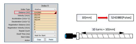
As you can see, movements by short distance like 1 [mm] and 10 [mm] can be made intuitively. However, to move the motor 5621 [mm], for example, we need a calculation.
