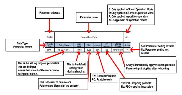
Parameters are categorized into immediately applied ones and ones that can be applied only if the servo power is turned on/off. The above table provides an example of the variable attributes.
