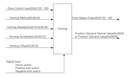
As shown in the figure below, you can set the offset between the home position and the zero position of the machine using the home offset function. The zero position indicates the point whose Position Actual Value (0x262A) is zero (0).
