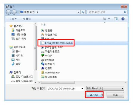
(7) Select the BIN file of the firmware to transmit and press the Open button.
