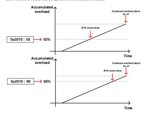
For example, when you input 50, W10 starts to occur at the point when accumulated overload becomes 50 [%]. If you input 90, it starts to occur at the 90 [%] mark. If accumulated overload becomes 100%, W10 is changed into AL-21.
