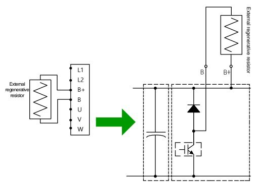
Wiring method for using external regenerative resistor
