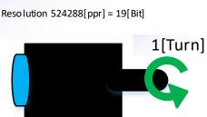
In this case, it is straightforward to enter a distance value to make 1 [turn] of a motor.
