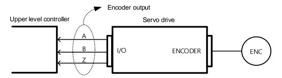
The encoder signal output frequency of the drive is 4 [Mpps] at the maximum for the line drive method.
