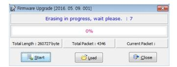
(9) Press the "Start" button to start transmission. A count-down of 10 seconds is activated to clear the internal memory in the drive. (Here, "Flash" is displayed for 7 segments for L7C.)
