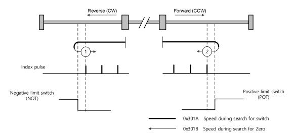
For homing using the homing method 1, the velocity profile according to the sequence is as follows. Refer to the description below.
