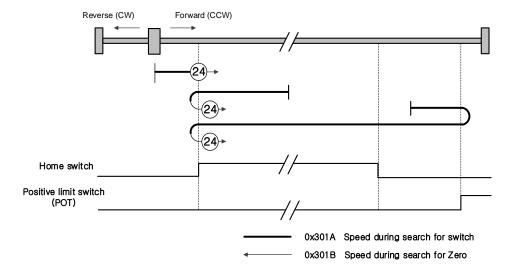
The initial driving direction is forward (CCW), and the point where the positive home switch is turned on becomes the home position.
