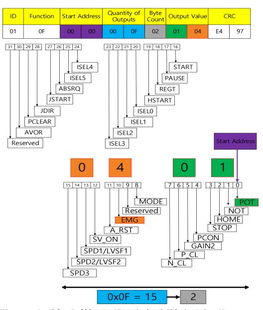
When you assign 15 Quantity Of Outputs while starting from 0x00 for the starting address, you can control the input up to 0x14. As the upper and lower Output Values are swapped, please be careful when you input them. When you input '01 04', for example, they will be swapped into '04 01'. 04 will turn on EMG, the 10th bit, and '01' will turn on POT, the Oth Bit.
