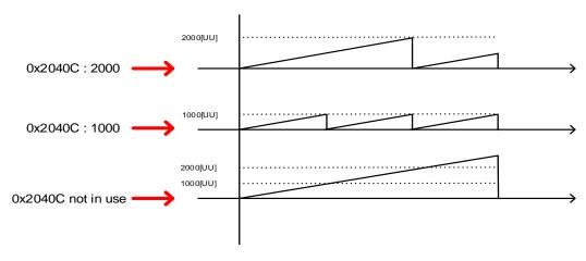
In general, when you do not use the Modulo factor, the current position keeps increasing when the motor rotates in one direction.
