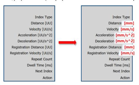
This is how we can change [UU] to [mm] for easier operation.
