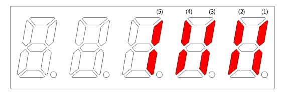
If an LED that corresponds to a contact is turned on/off, it indicates the ON/OFF state of the contact.
