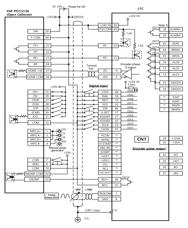
**X** This is an example of a wiring diagram for a single shaft. For wiring with 2 or 3 shafts, refer to the pin arrangement for the positioning module.
