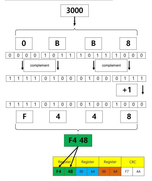
When you input -3000, 3000 is converted into a hexadecimal number first. The complement is taken and 1 is added to the 0th bit.
