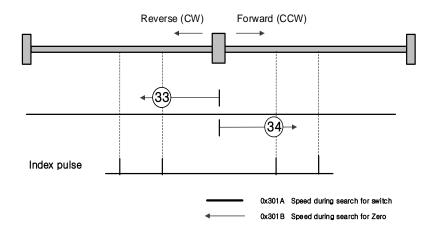
The initial driving direction is reverse (CW) for method 33 and forward (CCW) for method 34. The drive detects the index pulse at the zero search speed.
