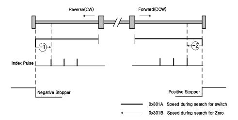
Homing method -1 and -2 perform homing by using the stopper and index (Z) pulse. The velocity profile according to sequence is as follows. For more information, see the details below.
