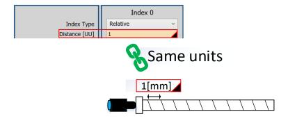
Thus, you just have to input 1 [UU] for Distance to move the linear motor 1 [mm].
