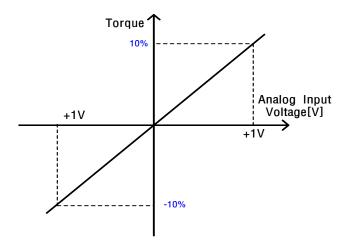
The related object is the 0x2210 analog torque input (command/limit) scale, which consists of two functions.
