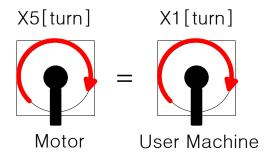
When the machine's apparatus makes 1 [turn], the total pulse required for the machine's 1 [turn] for the installed L7 19 [bit] motor's 5 [turn] is as follows.
