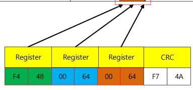
When you input -3000, "F4 48" is input in the register. The following example shows the conversion process. Refer to the example.
