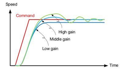
The value and the responsiveness have an inverse proportion relationship where a higher value results in a lower responding speed. Too high of the integral gain increases the overshoot. In this case, P/PI conversion can manage the overshoot.
