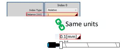
Here, the input distance unit becomes 0.1 [mm]. In the same way, if you need to make a movement of 0.01 [mm] or 0.001 [mm], you can enter a larger value into Electric Gear Denomiator 1[0x3010] to increase precision.
