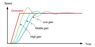
The higher the speed proportional gain value, the feedback speed's responsiveness to the command speed becomes better. However, if the value is too high, an overshoot or ringing may occur. In contrast, if the value is too low, the responding speed becomes low, which slows down system operation.
