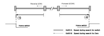
Homing methods -5 and -6 perform homing only by using the stopper. The velocity profile according to sequence is as follows. Homing is stopped when the drive meets the limit switch. For more information, see the details below:
