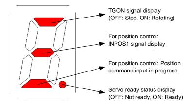
Digit 5 displays the current control mode status and servo on status.
