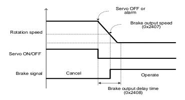
Timing diagram for signal output by the brake output speed (0x2407)
