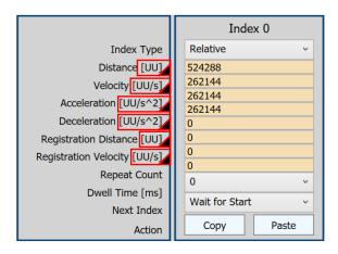
If gear ratio is not used, [UU] in the index is converted to [Pulses].
