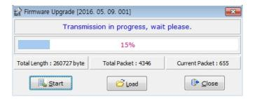
(10) After clearing, the firmware is transmitted automatically and the progress bar and "Current Packet" display the current transmission status. (The transmission time depends on the PC performance, but it usually takes from tens of seconds to several minutes.)
