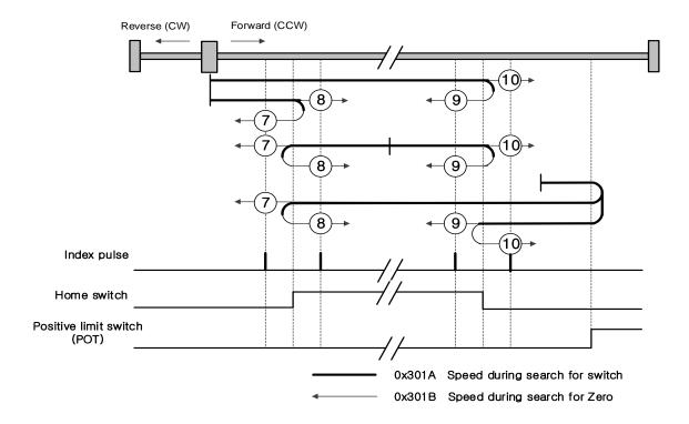
For homing using the homing method 7, the velocity profile according to the sequence is as follows. The sequence varies depending on the relationship between the load position and the home switch during homing, which is categorized into three cases as below. For more information, see the details below.
