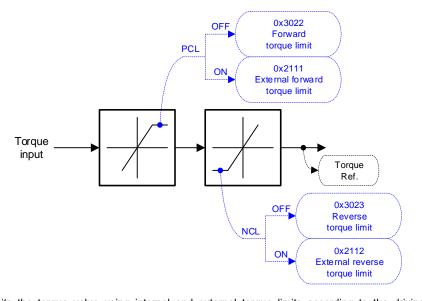
Internal + External Torque Limits
