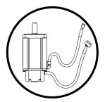
Do not pressurize or damage the cables. Make sure to use robot cables for a moving motor and prevent the cables from swaying.
