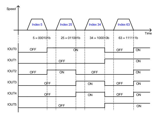
The current index position output signals are initialized when the operation mode is changed or the SVON signal is turned off (Motor free-run state). The initialized output state is identical to the operation status output of the number 0 index, which is why it is advisable to start with Index 1 whenever possible.
