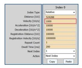
If you enter 1000 [UU/s] for index velocity, the motor runs at 3000 [rpm].
