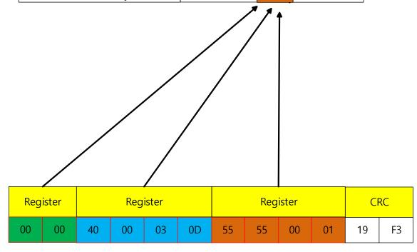
The number of registers differ for each parameter. To determine the value of Quantity of Register, find out the variable format on the communication address table. The register quantity is 1 for 16 [bit] and 2 for 32 [bit]. Add the values and input the result value. Input the value twice Quantity of Register for Byte Count.
